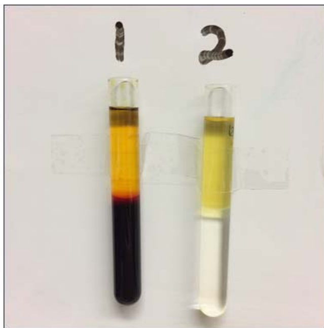
Fig 2. Iodine solution partitioned between water and ethyl acetate either (1) before or (2) after addition of sodium metabisulfite.
