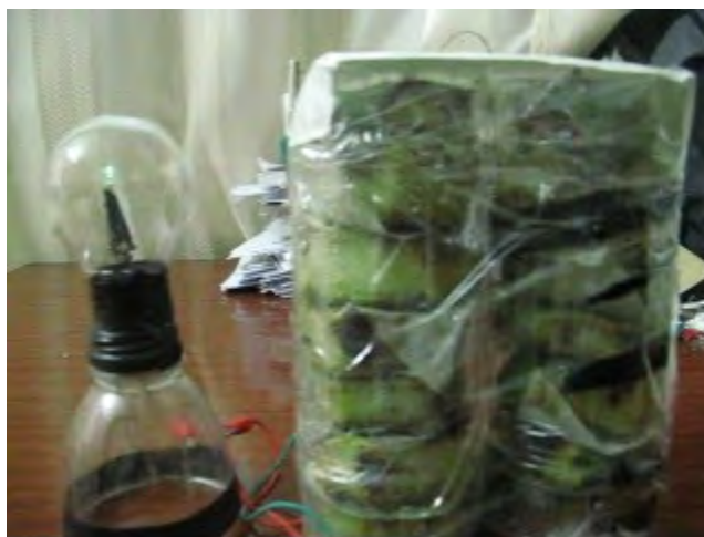
Fig 7. The Modified Form of the Cactus Battery by Using Two Plastic Bottles of Cactus Pieces Connected in Series by Using Mg/Cu Electrodes
