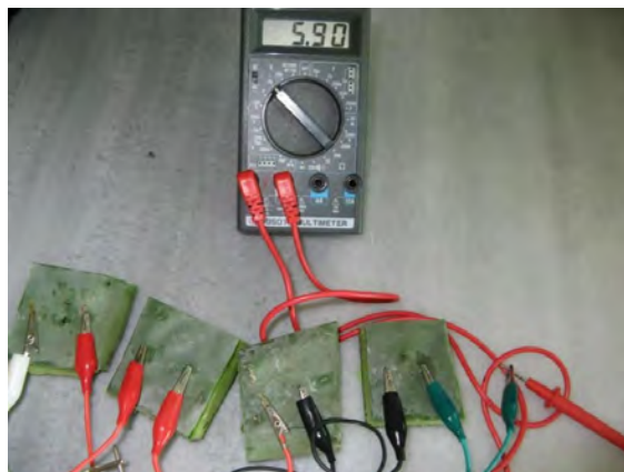
Fig 2. Potential Difference Measurement for 4 Pieces of Cactus Connected in Series
