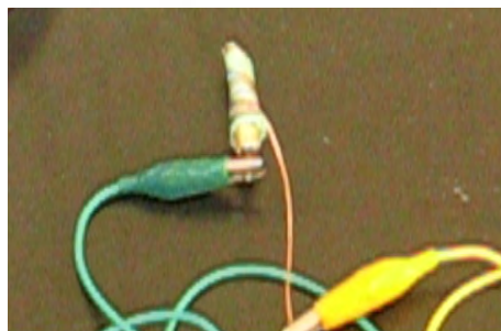
Figure 3. The Rolled Small-scale Galvanic Cell (Zn|ZnSO 4 (1.00M)||CuSO 4 (1.00M)|Cu)
